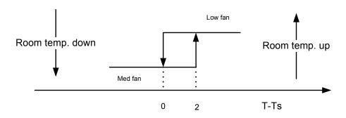
8.7.6 Indoor evaporator high-temperature protection at heating mode (T=indoor exchanger temp.)
